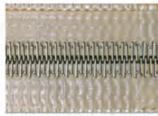
Clipper Splice Individual metal hooks are fastened to belt ends and joined together by a metal pin
